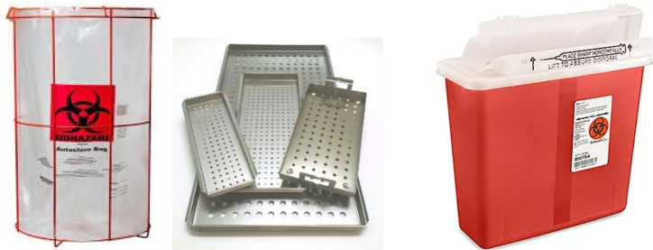
Left to Right: Autoclave bag in orange wire frame holder, autoclave trays, sharps bin
